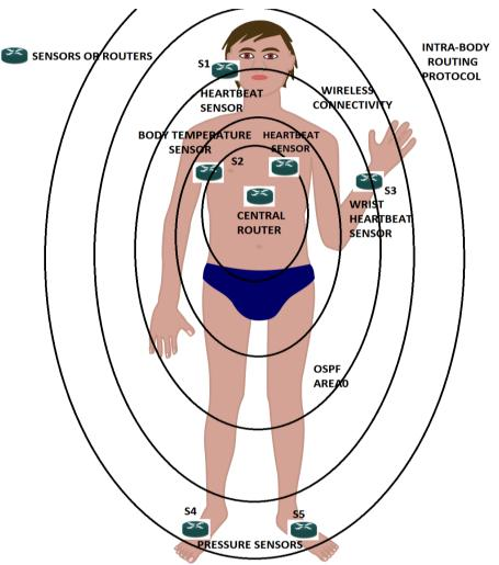
Figure 4 shows the placement of the sensors at strategic positions on the human body.
