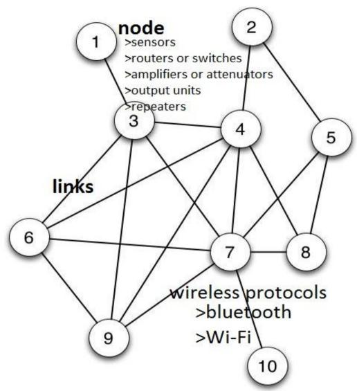
Figure 1 shows abstract nature of WBAN network consisting of nodes and links.
